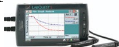
Temperature data - evaporation comparison with two stainless steel sensors
