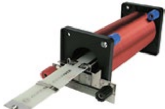
EM1230-001 Current Balance mounted on EM0090-001 Air Cored Solenoid
