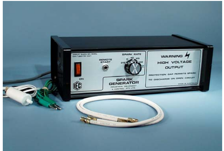
LB0118-001 Spark Generator & cables
