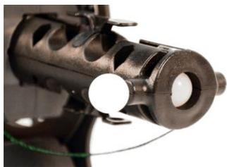
The accessory is now ready for use. The Launcher will fire the axial ball horizontally out of the device. As the ball leaves the chamber, the pin will retract and allow the drilled ball to fall vertically.
